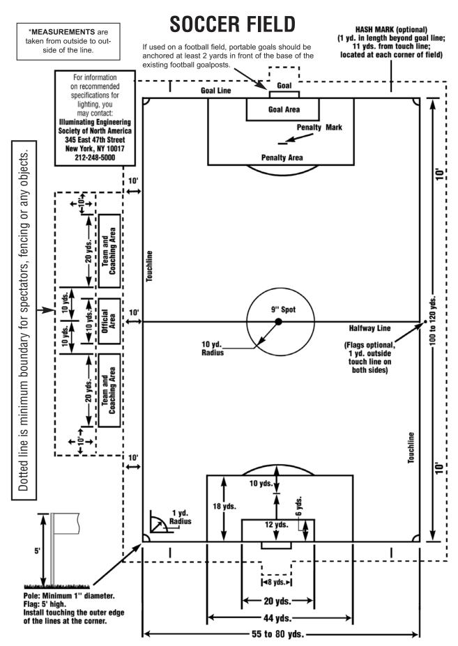
An engineered soccer field should have a minimum of one-and-one-half percent slope on fields which are surface drained and made up of native soil. For fields with underground drainage the slope should be no less than one percent slope. Slope is measured from center to side. Under no circumstances should a soccer field be flat. For more information, contact Design Architects, 816-842-5200.
